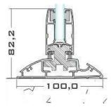
**Bifold Flat** The ramp profile provides isolation and easy passing with a threshold height of 23.3mm
