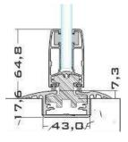
**Bifold Zero** An embedded railing profile, with a threshold height of 7.3mm
